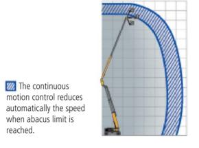
3 simultaneous and proportional movements: lifting, telescoping and turret rotation.
