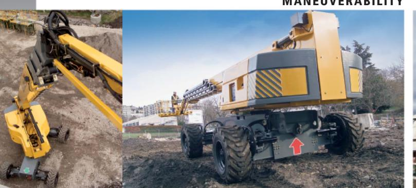
4-wheel drive and steer, coupled with the smallest turning radius in the market(1), allow for operation in a wide range of areas.
